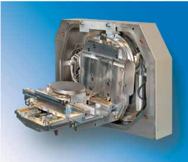
5-axes-manipulator for scanning electron microscopes SEM (X-, Y- and R-axes driven by Piezo-motors)
